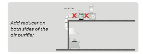
Install the fan on the air outlet, make air purifier work under negative pressure
